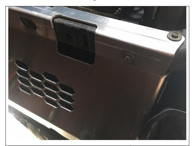
5. Reuse factory hardware and secure front of plate to cross member.
