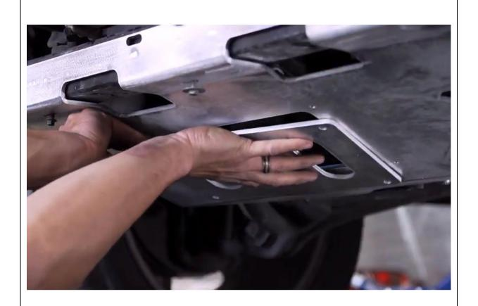
7. Fit cover panel with M6 button head cap screws and washers.
